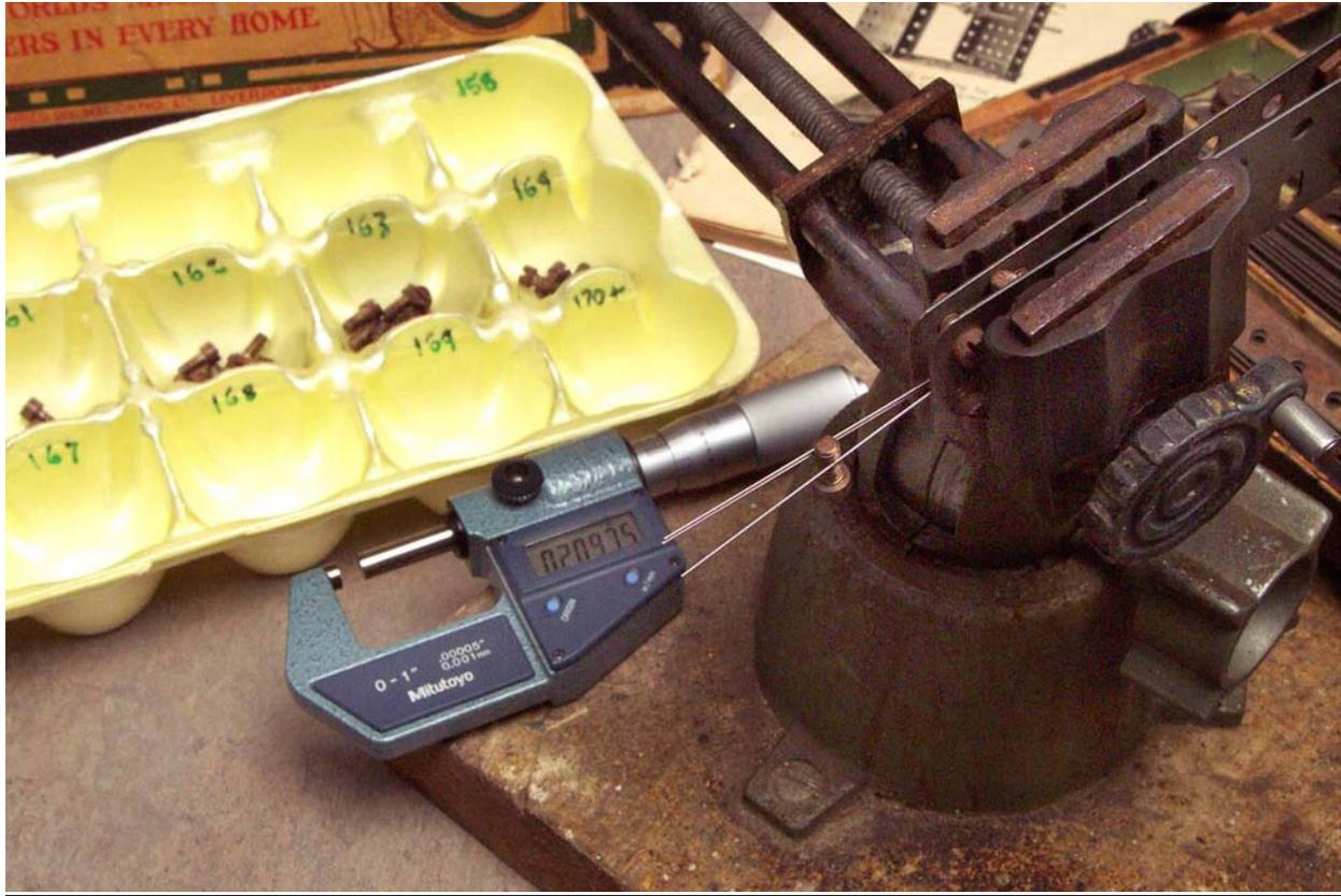
This is a view of the way I measured the bolts. The three wires are mounted in a holder made from two Flat Girders (tin plated, and so made in USA) and a 1" Threaded Rod. The holder is supported in a small vice. A bolt is shown supported by the wires, ready for a measurement. The egg carton, with the sized marked, is in the background.
